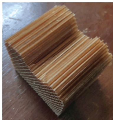
图20 超声插切加工曲面轮廓边界实物 Fig.20 Practicality of ultrasonic slotting curve edge
